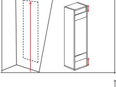
Make sure that there are no hidden pipes or cables in the wall. Drill 2 holes per mounting bar, using an 8mm drill bit to a depth of 55mm.
